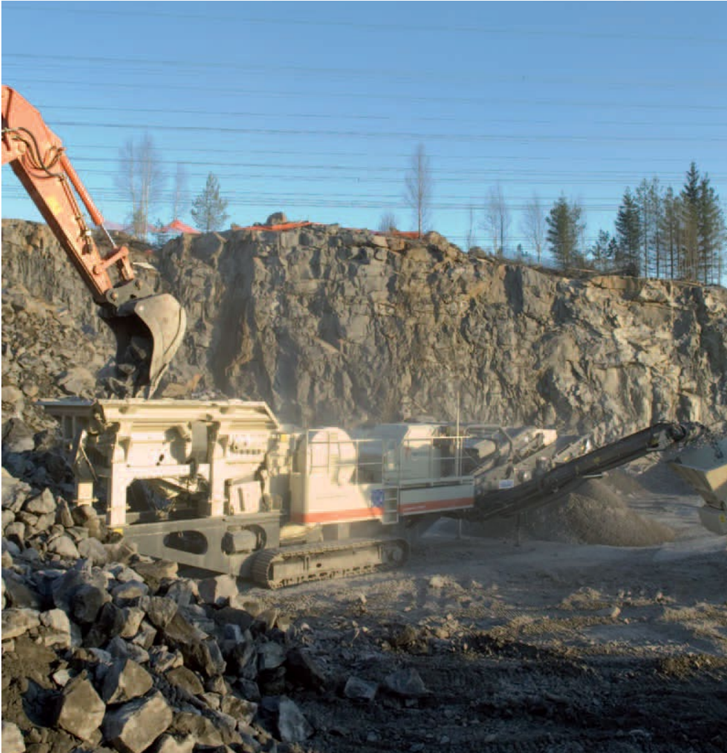
Illustration: Jaw crusher with integrated screen, working in quarry
