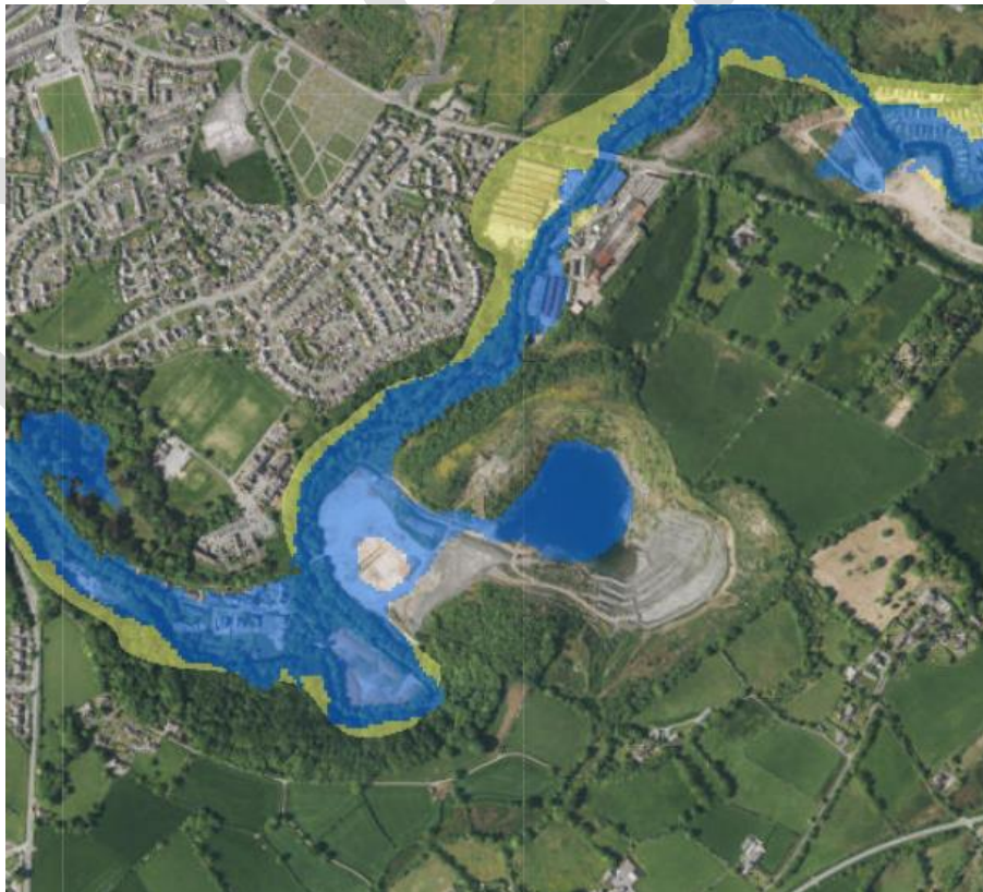
Figure 2.3 Extract of Development Advice Maps identifying extent of C2 flood area (in blue)
